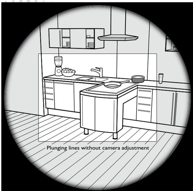
Plunging lines without camera adjustment
