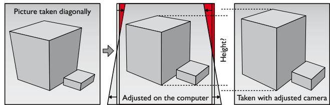
When adjusting a picture on the computer which has been taken with a fixed camera, the object will have to be changed into a trapezoid. Afterwards the picture will in turn have to be cut into a rectangle. The edges of the detail might get cut off in the process (see red). The picture would also have to be stretched lengthwise.
